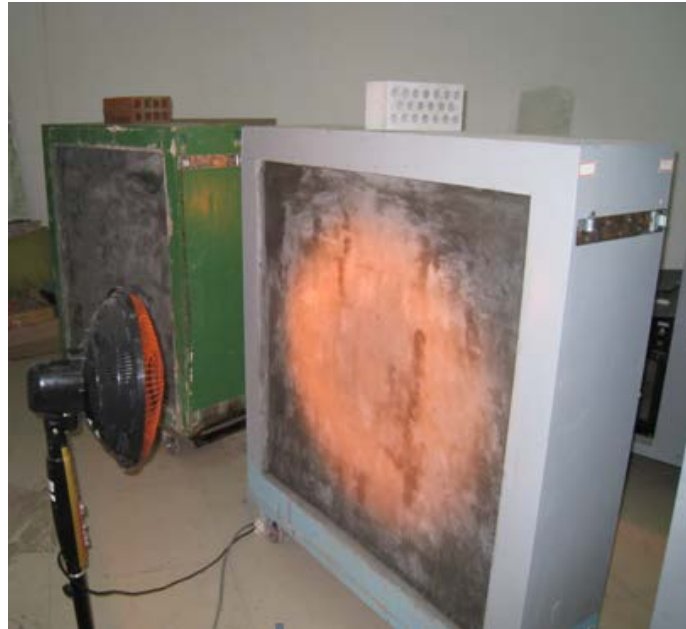
Figure 3. The test wall dried by warmer.
