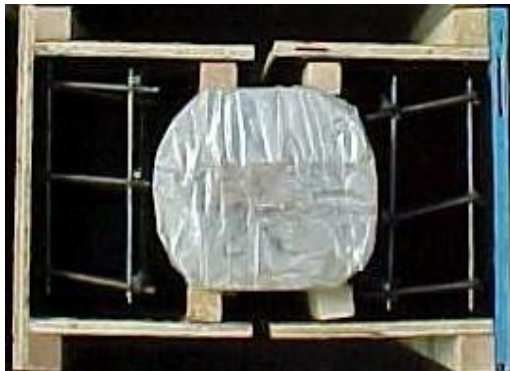
Fig. 4. Reinforcement details for the wood-concrete specimen
