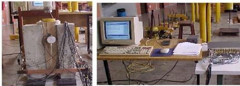
Fig. 5. Instrumented specimen details and data acquisition system
