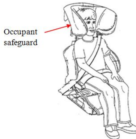
Fig. 25. Proposed design of child booster seat by Thomas Charles Baloga and Adrian Simms [31]
