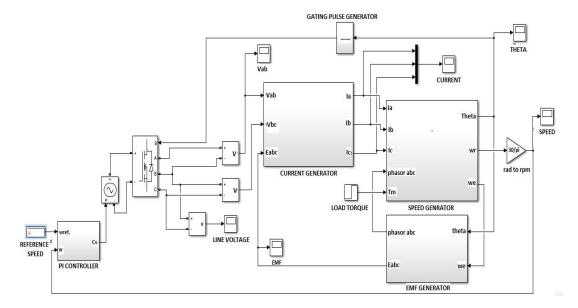
Fig. 6. Model of BLDC motor drive
