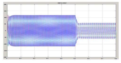
Fig. 9. Back EMF (y-axis) vs. time (x-axis)
