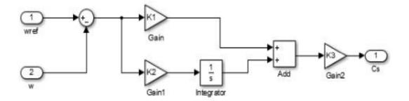
Fig. 3. PI controller with tunable parameter K1, K2 & K3
