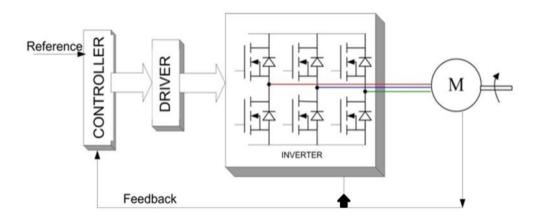
Fig. 1. BLDC motor control scheme
