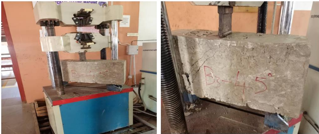
Plate 1. Loading of beams with 90° and 45.0° shear reinforcements
