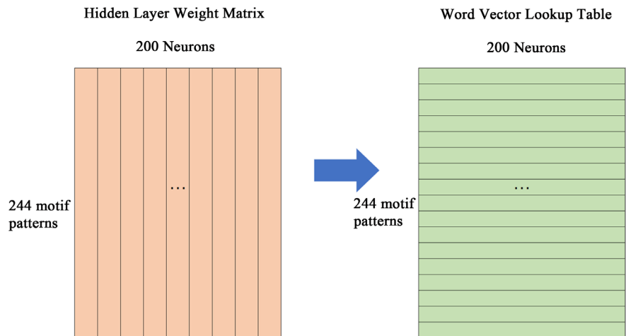
Figure 3. In the hidden layer weight matrix, each column represents the hidden layer neurons' weights of one motif pattern. In the word vector lookup table, each row represents each motif pattern in the vector space.
