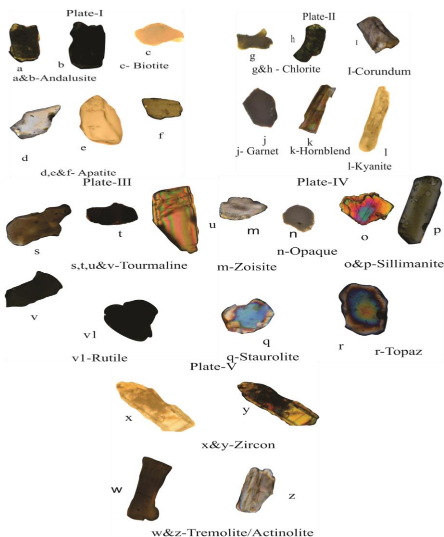
Fig. 4. Heavy mineral assemblage in ox-bow lake sediments of Ganga alluvial plain (Plate I-V)
