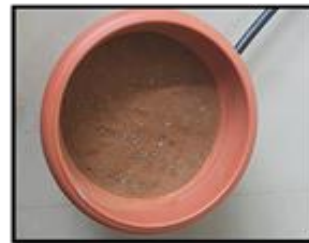
5. Filling a layer of soil
