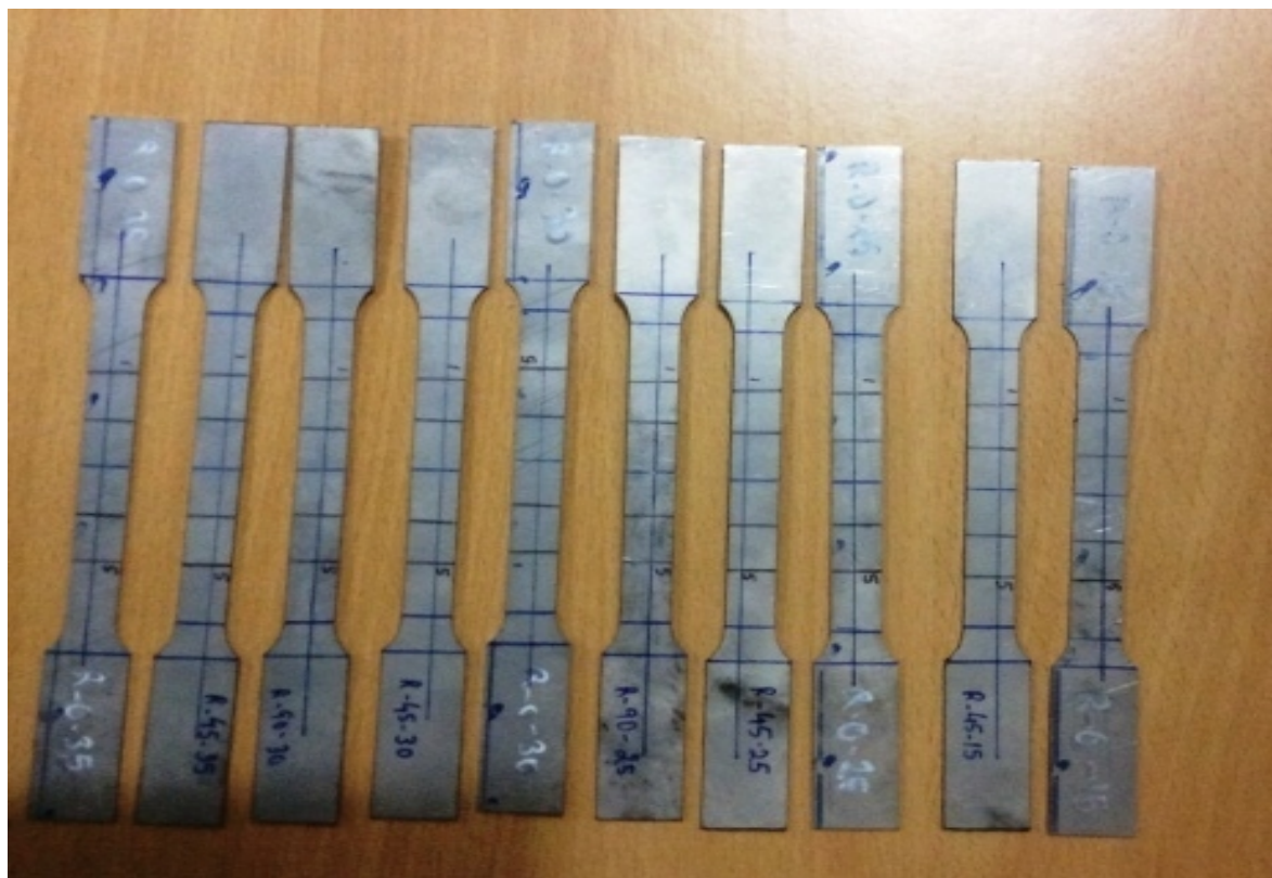
Fig. 1. Tensile tested specimens for determination of plastic strain ratio
