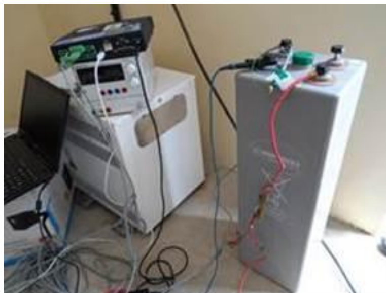
Fig. 4. Battery test assembly
