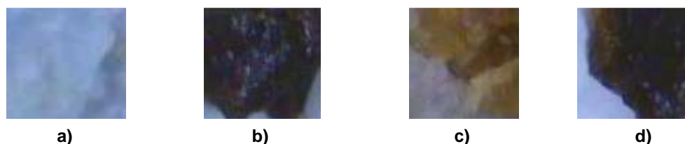
Fig. 2. Change in the state of the catalyst Cu(II)/PAAH in the presence of substrates: a) the starting sample, b) after treatment with 0.1 M sodium sulfide solution, c) after treatment with a 0.1 M cysteine solution, alkaline to pH 12.5, d) after treatment with a mixture of sodium sulfide and cysteine
