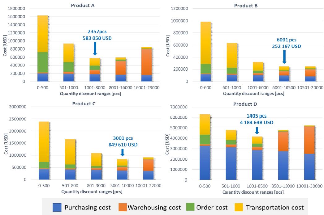
Fig. 2. Results of Scenario 1: conventional computation of economic order quantity with quantity discount and costs of transportation
