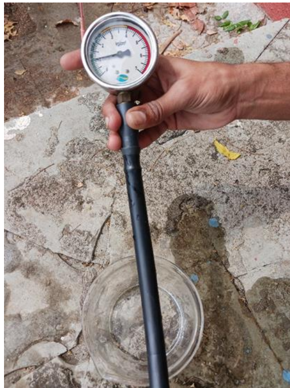
Fig. 2. Measurement flow of distinct emitter for calculation of manufacturer’s coefficient of variation
