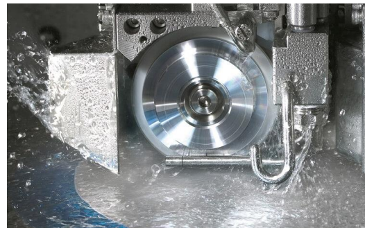
Fig. 1. Mechanical wafer dicing saw process [1]
